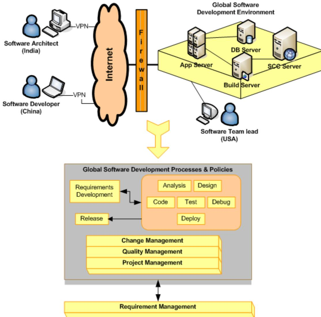
*The diagram shows software teams working in India, China, and US, the development environment is physically located in US. The global development environment shows a simplistic view of different servers connected together, other servers might exist in large projects. Each developer has an IDE that is connected to the development environment located in US that gives seamless global software development process and policies to the entire project team.*
